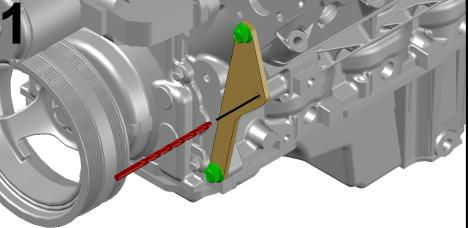
\*Optional, for more rigid mounting - if using an iron (truck) block, drill boss with letter "R" drill and use M10-1.5 tap. Drill Template (551445) shown above - NOT INCLUDED
