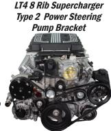
Add a hydraulic power steering pump to your Gen 5 LT4 engine with this power steering kit. Requires the use of a 2010-2012 LS3 Camaro power steering pump, Retains factory LT4 accessories. ParNumer Price
