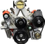
Billet aluminum brackets place the alternator and power steering pump in the factory configuration of an LS1. Requires the use of a 98' to 02' F-Body Camaro power steering pump. Will work with any LS alternator except Corvette. Available for Truck or Camaro spacing
