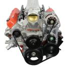
Replaces the large cast factory truck accessory bracket and re-uses your factory Alternator and Power Steering Pump. Part Number Price
