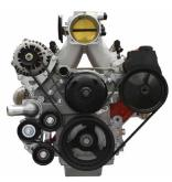
This Kit places the alternator and power steering further inward than other kits to provide clearance for forward facing turbo manifolds. Requires 105 amp alternator and a 98'-02' Camaro power steering pump.
