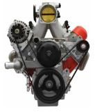
This kit places the alternator further in than other kits to provide clearance for forward facing turbo manifolds. Requires 105 or 145 amp alternator, LS1 water pump, and includes a manual belt tensioner mounted on the drivers side head.
