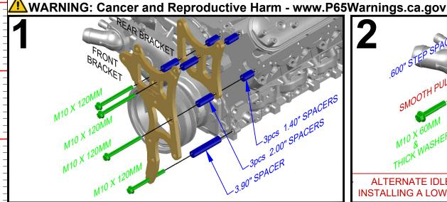
ALTERNATE IDLER PULLEY POSITION USED IF INSTALLING A LOW PROFILE INTAKE (LS1, LS3, LS6)
