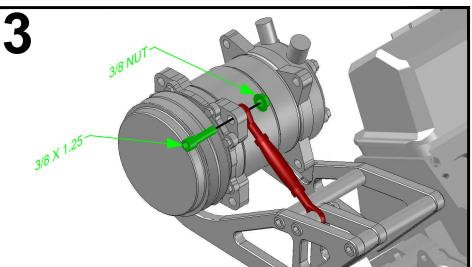
**INSTALL BELT WITH** TENSIONER AT SHORTEST LENGTH. SET BELT TENSION BY TURNING TENSIONER **COLLAR WITH WRENCH**
