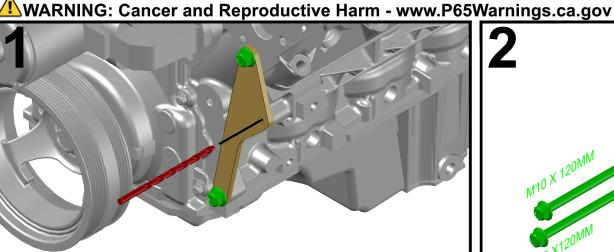
\*Optional, for more rigid mounting - if using an iron (truck) block, drill boss with letter "R" drill and use M10-1.5 tap. Drill Template (551445) shown above - NOT INCLUDED
