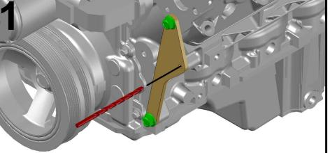
\*Optional, for more rigid mounting - if using an iron (truck) block, drill boss with letter "R" drill and use M10-1.5 tap. Drill Template (551445) shown above - NOT INCLUDED
