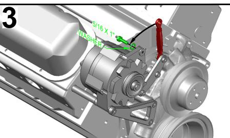
INSTALL BELT WITH TENSIONER AT SHORTEST LENGTH. SET BELT TENSION BY TURNING TENSIONER COLLAR WITH WRENCH
