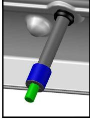
PRE-INSTALL BOLT, WASHER, SEAL, RISER, RISER SPACER, AND RETAINING PUSH NUT INTO VALVE COVER PRIOR TO INSTALLING VALVE COVER SPACER AND VALVE COVER ONTO CYLINDER HEAD
