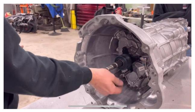
2. Mark the 2<sup>nd</sup> rib back from the bellhousing mating surface to begin cutting off the old bellhousing.
