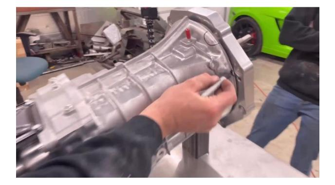
7. After marking where to notch, reinstall the bearing plate temporarily to keep debris out while you make your cut/notch.
