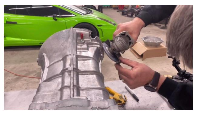
9. Remove the bearing plate for the final time and clean the mating surface so the RTV will adhere.
