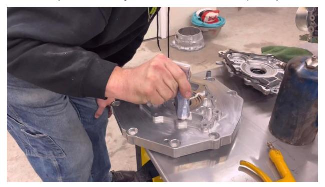
12. Use the supplied allen bolts to mount the adapter to the transmission. Apply RTV around the treads of the bottom 4 bolts as they are submerged in fluid at all times.
