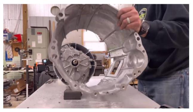
5. Clean up the area where you cut so none of the housing interferes with the adapter, and to remove sharp edges that could slice a limb off.
