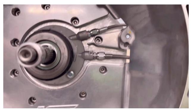
15. Install the GM bellhousing with supplied fasteners and torque to 40 ft-lb.
