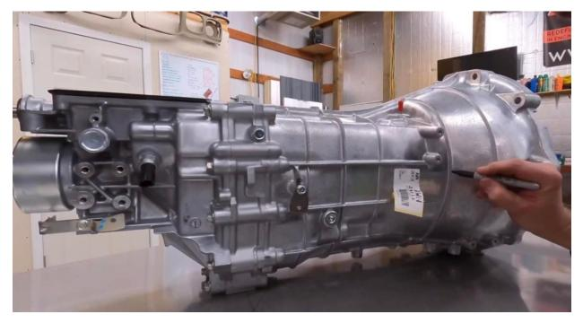
3. Begin cutting the bellhousing off. Be carful not to cut to deep into the bearing plate/adapter housing.
