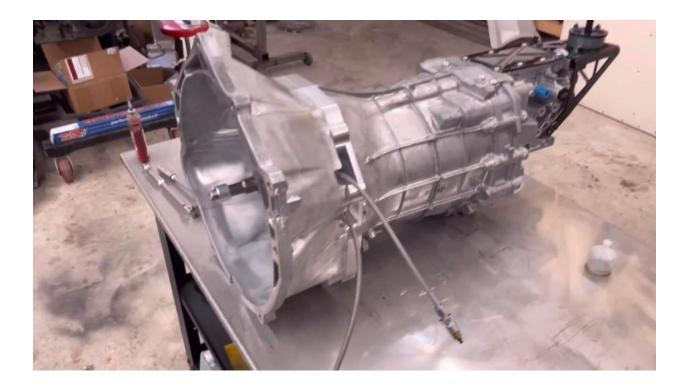
Thank you for purchasing ICT Billets CD/JK bellhousing adapter kit. These instructions will guide you though the process of removing your old bellhousing, prepping the transmission for the ICT Billet adapter, and installing the adapter and GM bellhousing.
