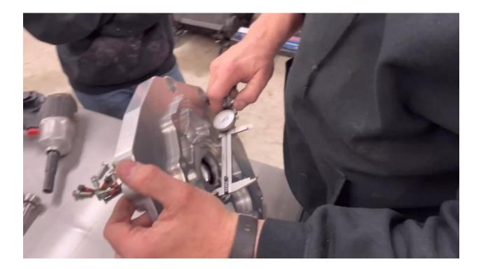
11. Once you have verified that you have the correct adapter, clean the mating surface and apply Ultra Grey RTV around the outside perimeter, then slide it on the transmission. **This adapter does not use a gasket between the case and the adapter, only RTV**.
