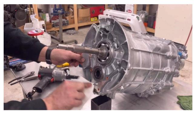
10. Before you mount your adapter, be sure to measure the main bearing diameter just to make sure you have the correct adapter. It's the second step of the bearing retainer and the adapter.
