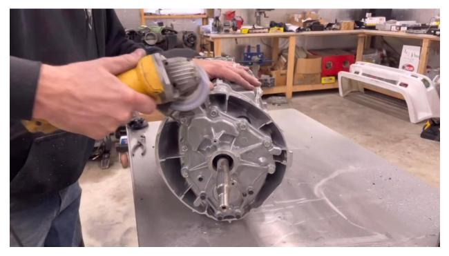
6. Remove the bearing plate to test fit the adapter and mark where to notch for your trans to bellhousing bolts.
